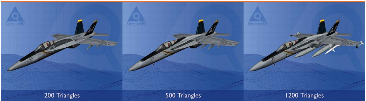
Quantum3D® Facets® Realtime 3D Models with 3 Levels of Detail Shown
