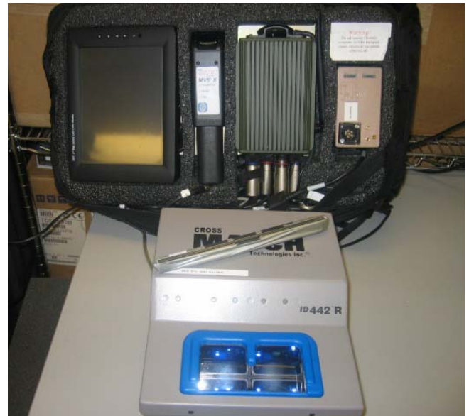
U.S. Navy EMIO Identity-Data Toolset Rapid-Deployment Capability Program Based On Cross Match® Multi-Modal Jump Kits That Include a Quantum3D® Thermite® TVC-2.0 Model 1010 with GPS Receiver, Fingerprint Scanner and Display with User Interface, Waterproof Backpack and Cable Assemblies Photo Courtesy U.S. Navy
