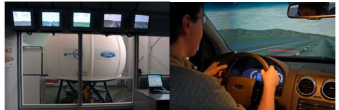
Ford Motor's VIRTTEX Simulator is a 24-foot diameter dome with six hydraulic actuators and six degrees of freedom, enabling the driver to experience a realistic driving simulation. (Photos Courtesy of Ford Motor Company)
