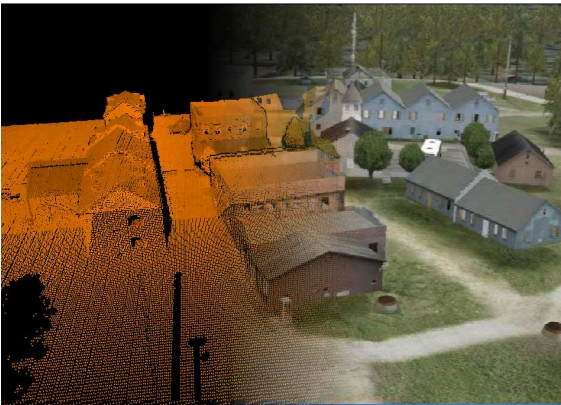
CG 2 artist rendering of path of unprocessed LIDAR data points (left side) to visual database product (right side).
