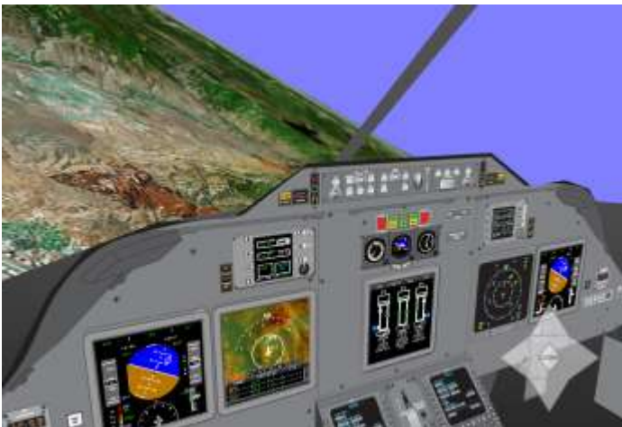
IData 3.0.4 demonstration shows new ARINC 661 compliant widget library, IData3D UI widgets, and TerraMetrics whole-earth satellite imagery TerraBlocks terrain rendering integrated with IData3D.
