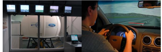
Ford Motor's VIRTTEX Simulator is a 24-foot diameter dome with six hydraulic actuators and six degrees of freedom, enabling the driver to experience a realistic driving simulation. (Photos Courtesy of Ford Motor Company)
